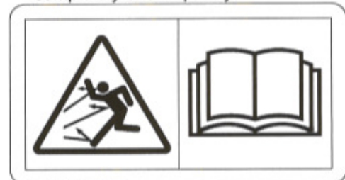
(4) Part No. V0511-5764-1 [Both sides] Do not loosen the grease nipple completely or too quickly.
