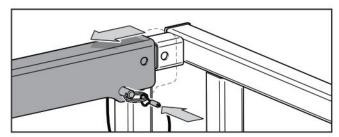
**15.** Remove the **lock-pins** on the top rear gate.
