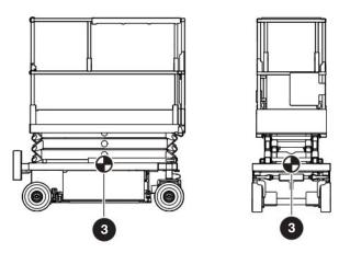
Figure 18 Center of gravity
