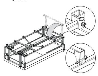
Fold the guardrails Section 6 – Procedures
