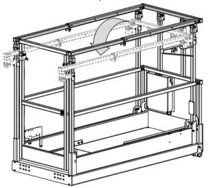
Section 6 - Procedures Fold the guardrails
