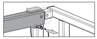
14. Remove the lock-pins on the top rear gate.
