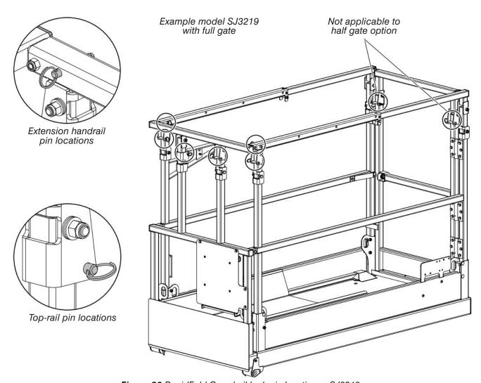
Figure 26 RapidFold Guardrail lock-pin locations - SJ3219
