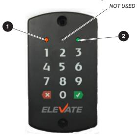
Figure 06 Keypad of the access control unit
