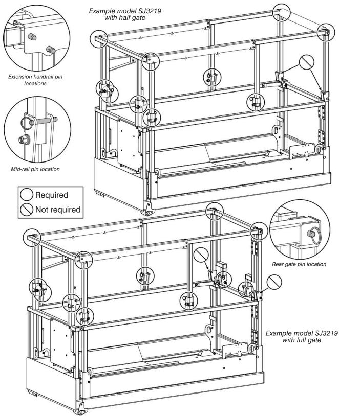
Figure 19 Guardrail lock-pin locations - SJ3215, SJ3219, SJ3220, SJ3226
