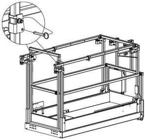
16. Hold the vertical bar of the entrance guardrail with one hand, and then fold the entrance top-rail with the other hand
