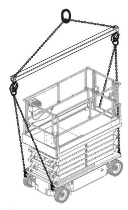
Figure 16 Appropriate method to hoist
