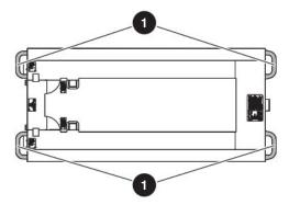
Figure 15 Lift and tie-down points
