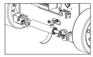
Figure 13 Brake release block (pin brakes)
