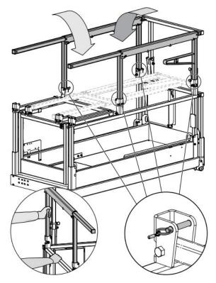
Figure 23 Left and right guardrail folded
