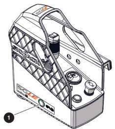
**1 SGLE:** This push-button energizes the lift function. Hold the button down together with the functionenable switch to enable the raising of the platform with the lift function.
