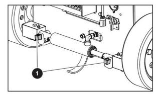
Figure 02 Brake release block (pin brakes)
