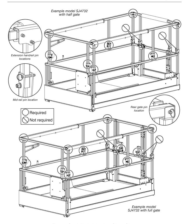
Figure 20 Guardrail lock-pin locations - SJ4726, SJ4732
