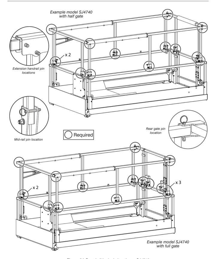
Figure 21 Guardrail lock-pin locations - SJ4740
