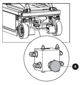
Figure 04 Freewheeling valve (SJ3215 and SJ3219)
