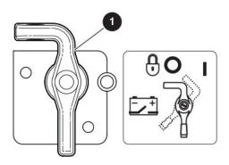
Main power disconnect: This switch disconnects power to all control circuits when in the off position. The switch must be in the on position to operate the MEWP. The switch must be in the off position when you transport the MEWP or put it in storage.
