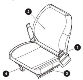
**1** Seat Belt: The operator's seat is equipped with a seat belt. Use this seat belt at all times when operating telehandler.
