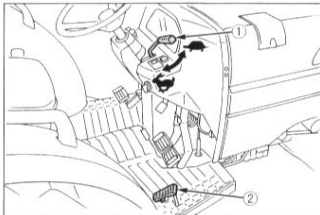
(1) Hand throttle lever ↗ "INCREASE" (2) Foot throttle ↘ "DECREASE" [except HST Type]
