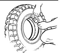
NOTE: If the wheel rim width is less than six inches, the TBS will contain one valve hole to accommodate the needle valve. If the wheel rim width is greater than six inches, the TBS will have two holes for the needle valve.
