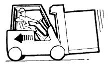
**4.** When traveling up or down grades in excess of 5% with a heavily loaded lift truck, keep the load upgrade to maintain control.
