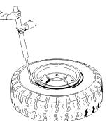
**2.** Put the tire tool into the slot between the lock ring and wheel rim. Remove the lock ring and side flange. If there is a flange seat, remove it.
