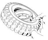
3. Turn over the rim and tire. Put. blocks under the rim so that the rim is 8 to 10 cm (3 to 4 in.) above the floor. Install the flange seat (if used) and the lock ring.
