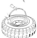
**4.** Put the lock ring in the correct position on the rim. Add air pressure to the tire as described in Add Air to Pneumatic Tires With Tube.
