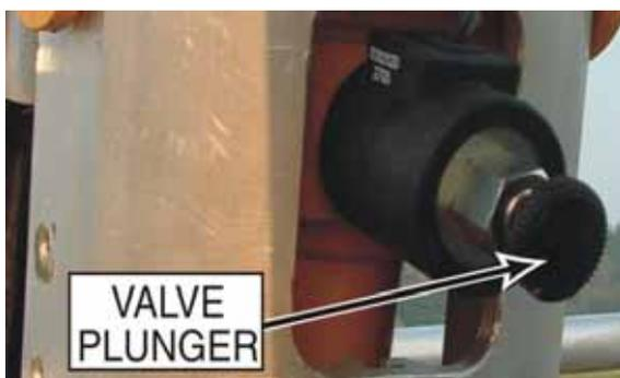
Figure 3-6. Manual Lowering Valve (Jib)
